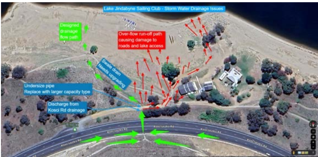
Fig 1. Aerial view of drainage flow paths causing ongoing damage to driveway and foreshore. Needs improving.
